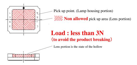
Please adjust the load, the pick up point, the nozzle diameter, etc. before mounting because the over load can cause the breakage of the lamp housing.
