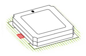
Recommended solder temp. measurement point
